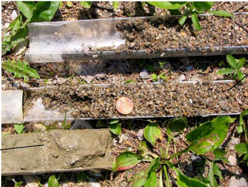
Figure 3: A.) Installation of piezometer cluster P2 using a Geoprobe™ direct-push machine. B.) Aquifer materials from P1L2, above 32 ft (silt) and below 32 ft (coarse sand).
